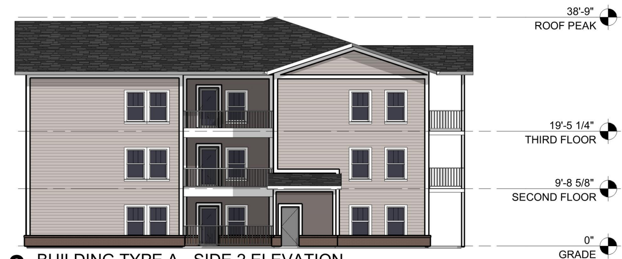
3 BUILDING TYPE A - SIDE 2 ELEVATION 1/16" = 1'-0"
