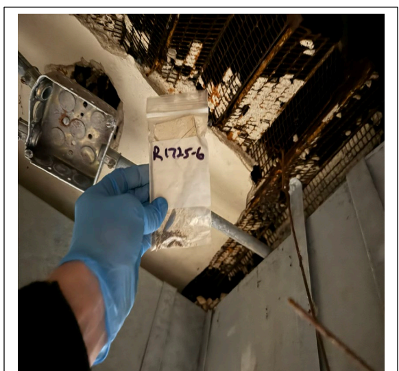
Sample R1725-6: Plaster (paint) from west building basement negative for asbestos.
