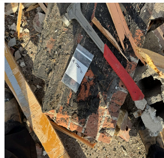
Sample R1925-10: Tar on parapet wall, (debris) from SW addition from larger building negative for asbestos.
