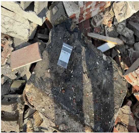
Sample R1925-7: Tar on parapet wall, (debris) from SW addition, from larger building negative for asbestos.
