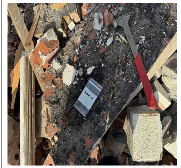
Sample R1925-11: Tar on parapet wall, (debris) from SW addition from larger building negative for asbestos.
