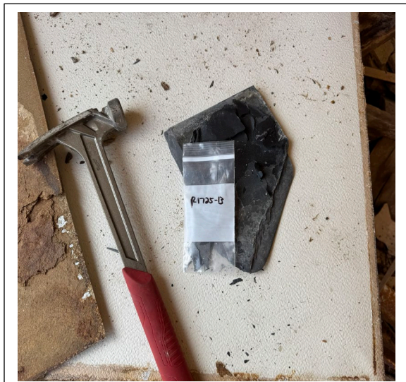
Sample R1925-13: Chalk boards from SE classrooms larger building negative for asbestos.
