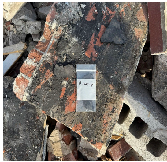
Sample R1925-8: Tar on parapet wall, (debris) from SW addition from larger building negative for asbestos.
