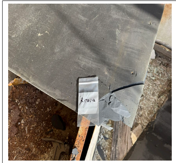
Sample R1925-12: Chalk boards from SE classrooms larger building negative for asbestos.
