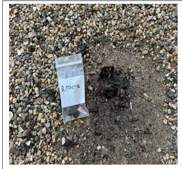
Sample R1925-16: Field from NW lower roof, larger building, negative for asbestos
