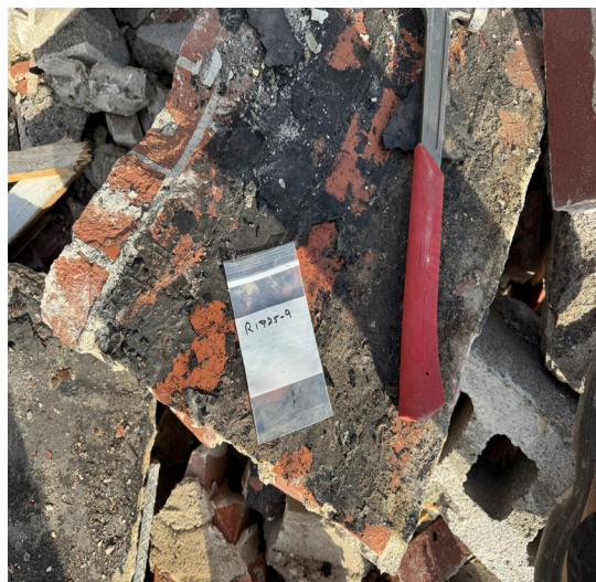
Sample R1925-9: Tar on parapet wall, (debris) from SW addition from larger building negative for asbestos.
