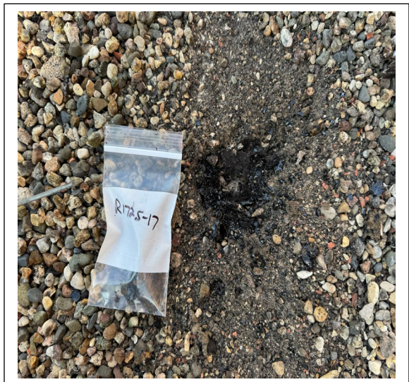
Sample R1925-17: Field from NW lower roof, larger building, negative for asbestos.
